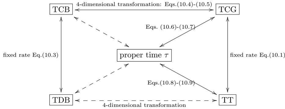
Figure 10.1: Various relativistic time scales and their relations. Each of the coordinate time scales TCB, TCG, TT and TDB can be related to the proper time  $\tau$  of an observer, provided that the trajectory of the observer in the BCRS and/or GCRS is known. Transformations shown as dashed lines are not explicitly described in this document.
